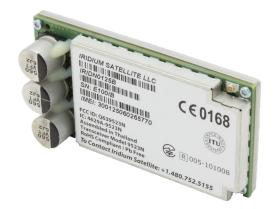
The Iridium<sup>®</sup> Core 9523 advanced voice and data satellite transceiver module is small, light and powerful. Its compact footprint and simple connections offer our partners new opportunities to integrate Iridium directly on their printed circuit boards (PCB) and develop products that meet the needs of previously unreached consumer and vertical markets like never before.
