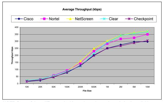
NOTE: Some of these differences in this graph are due to the variation in available bandwidth on the standard IP data connection. Thus, this graph alone cannot be used to determine which VPN is the most efficient over the BGAN network.
