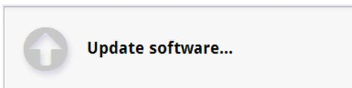
6. Browse to the new software version and click Open. The software file has the extension ".tiff". The EXPLORER 540 will upload the file and start updating the software.
